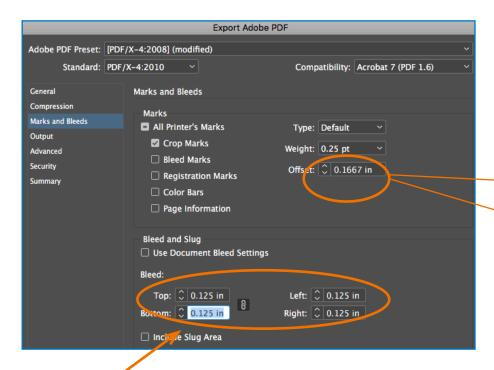
When saving the preset for offset measurement, enter 0.166665. The application view will default to only 4 numeric values behind the decimal however the actual number entered will hold.
